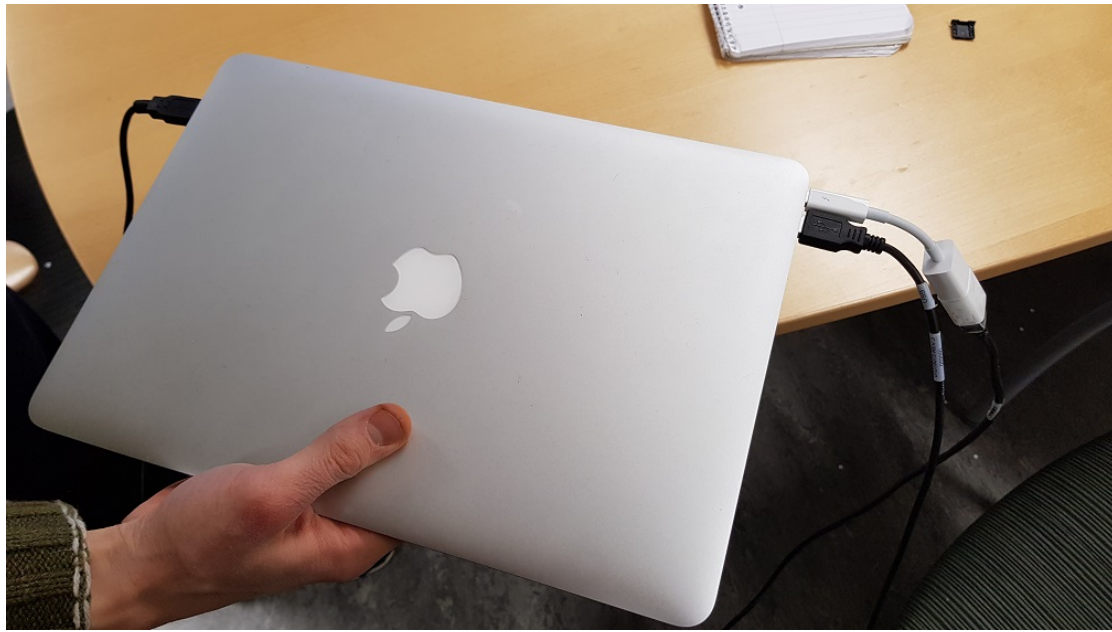
Figure B1.5 – Displays the proper sockets to use for connecting the Arduino (black USB, left in figure), INS (black USB, right in figure) and laser scanner (white Thunderbolt to Ethernet adapter, right in figure) to the computer.
