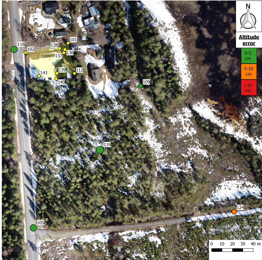
Figure 5 – A map of the GCPs (yellow dots) in the set of "Yard" when the image position is used, along with their covered area (1 094 m 2 ) and the CPs. The size of the CPs represent the combined error in Easting and Northing while the colour represent the error in Altitude as the scale on the map shows.
