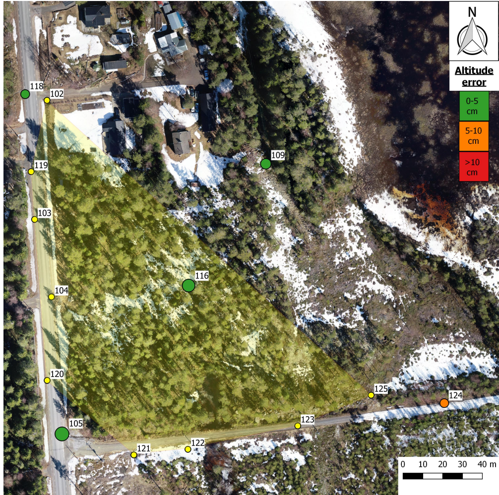
Figure 9 – A map of the GCPs (yellow dots) in the set of "Tarmac and gravel road" when the image position is used, along with their covered area (15 476 m 2 ) and the CPs. The size of the CPs represent the combined error in Easting and Northing while the colour represent the error in Altitude as the scale on the map shows.
