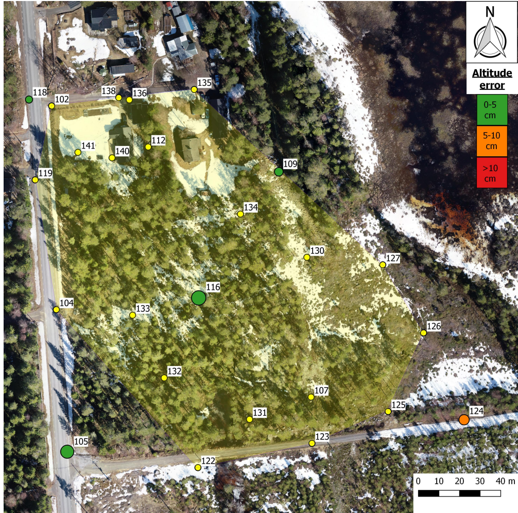
Figure 13 – A map of the GCPs (yellow dots) in the set of "Half of the GCPs" when the image position is used, along with their covered area (22 754 m 2 ) and the CPs. The size of the CPs represent the combined error in Easting and Northing while the colour represent the error in Altitude as the scale on the map shows.
