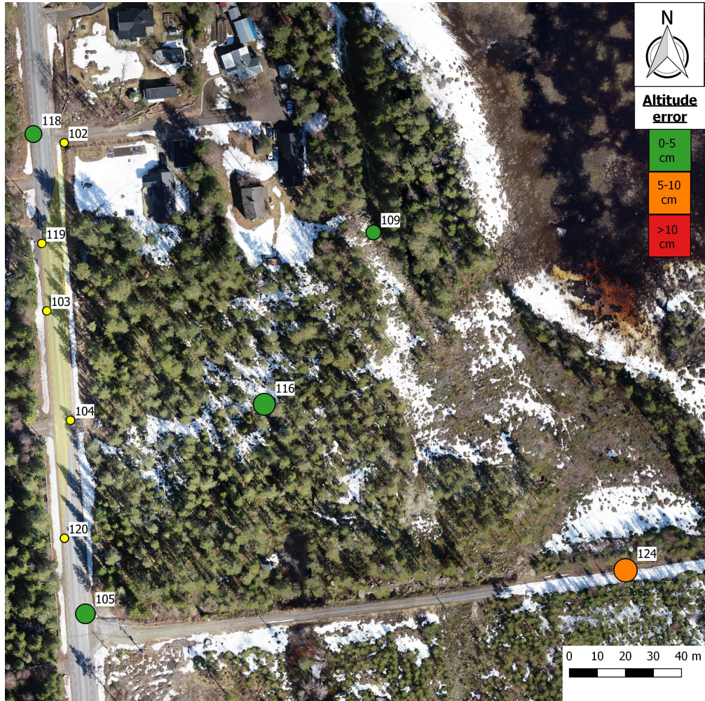
Figure 4 – A map of the GCPs (yellow dots) in the set of "Tarmac road" when the image position is not used, along with their covered area (763 m 2 ) and the CPs. The size of the CPs represent the combined error in Easting and Northing while the colour represent the error in Altitude as the scale on the map shows.
