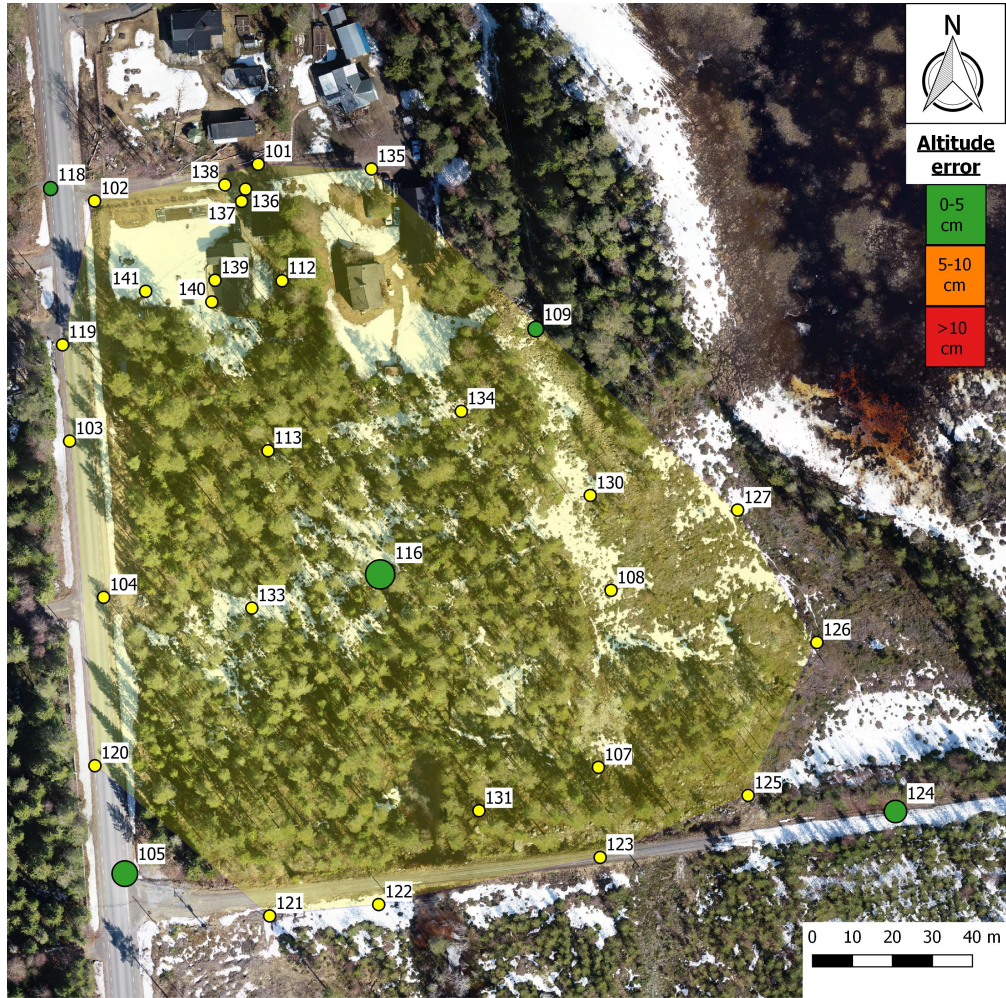
Figure 16 – A map of the GCPs (yellow dots) in the set of "All GCPs" when the image position is not used, along with their covered area (22 754 m 2 ) and the CPs. The size of the CPs represent the combined error in Easting and Northing while the colour represent the error in Altitude as the scale on the map shows.
