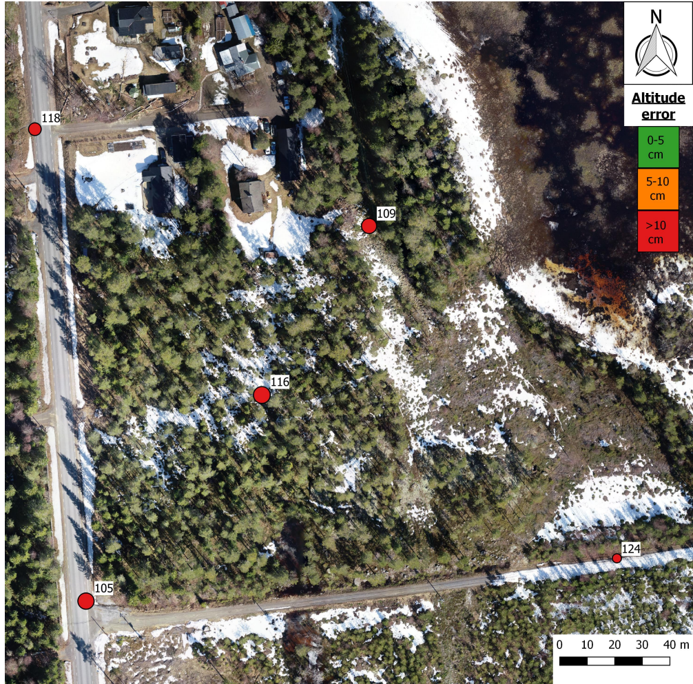
Figure 2 – A map of the set of "No GCPs" when the image position is used, with the CPs. The size of the CPs represent the combined error in Easting and Northing while the colour represent the error in Altitude as the scale on the map shows.
